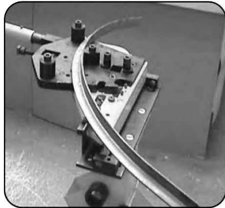
The key to achieving nice smooth curves is to bend gradually and consistently.
