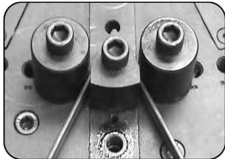
In position 1 it is possible to create bends as tight as 60° in one pass
