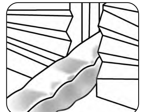
Applying gentle curved indents down the length of the tube achieves a decorative hammered effect.
