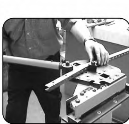
Channel or 'T' bar can also be curved using this process - this would be difficult to achieve by any other method.
