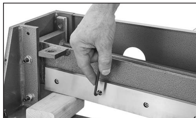
Figure 16. Use a wood block to keep blade from dropping during the removal process.
