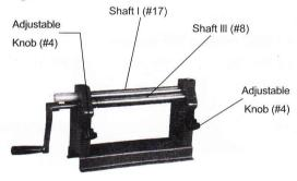
Figure 2-Adjusting the Roll Gap
