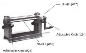
Figure 1-Adjusting the Material Gap
