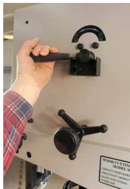
The doors are micro-switched but the bandwheels are not braked
