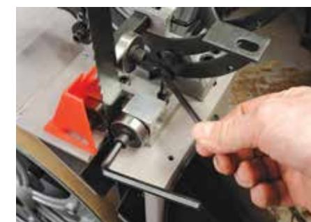
Showing how the guides are adjusted – table removed
