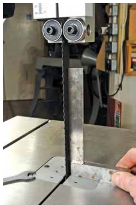
Checking the table is perpendicular to the blade
