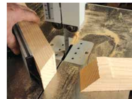
Making a mitre cut with the handy protractor
