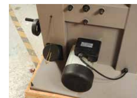
The lower dust port is capped but should be used ideally
