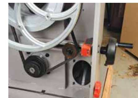
The pulley tensioning handwheel
