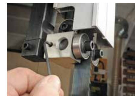
All guide adjustments are done with an Allen key
