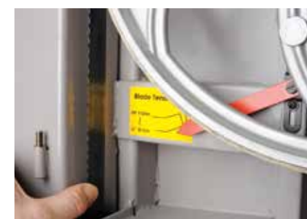
Flicking the blade to assess the level of tension
